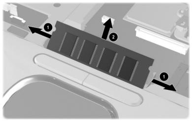
Removing an Internal Memory Expansion Board
